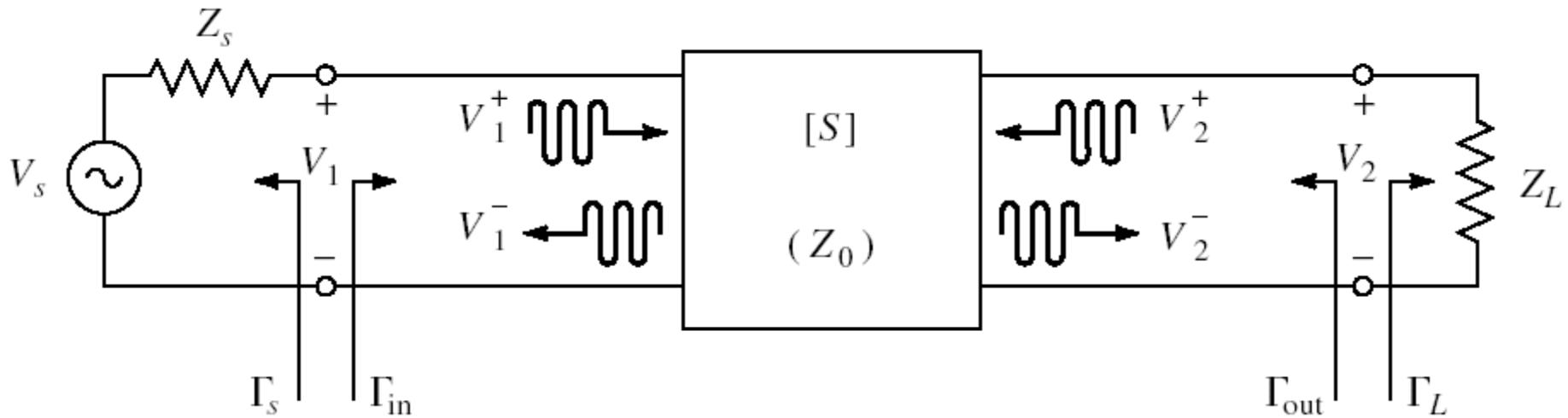
$$V_1^- = S_{11} \cdot V_1^+ + S_{12} \cdot V_2^+ = S_{11} \cdot V_1^+ + S_{12} \cdot \Gamma_L \cdot V_2^-$$
